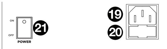
**19. Power Cable Input (IEC):** Insert the included power cable here to power the unit.
