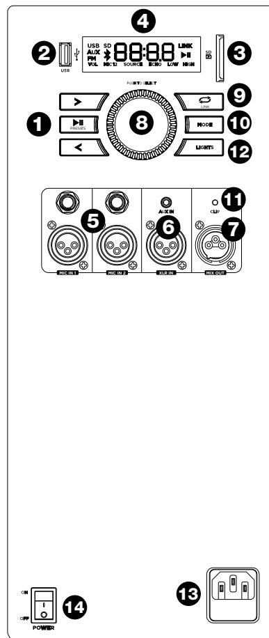
11. **Clip LED:** The Clip LED will flash red if the signal from the input jacks or **Media Panel** audio source is clipping (distortion from an overly loud signal). If this happens, decrease the setting of the **Main Volume** knob or the volume for the **Aux/Mic Input** (if a loud device is plugged into either).
