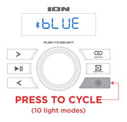
Press the **Light** button to toggle between one of the modes for the LEDs on Total PA<sup>™</sup> Titan.
