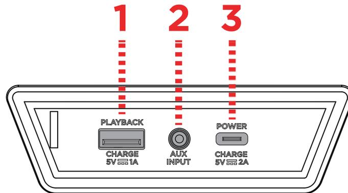
**Note:** Pull the tab on the protective rubber panel to release it and access the rear panel ports.
