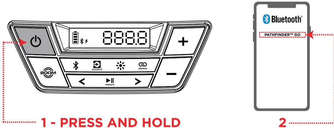
1. Turn on Pathfinder™ Go by holding down the **Power** button for 2 seconds. Pathfinder™ Go will automatically enter Bluetooth pairing mode.
