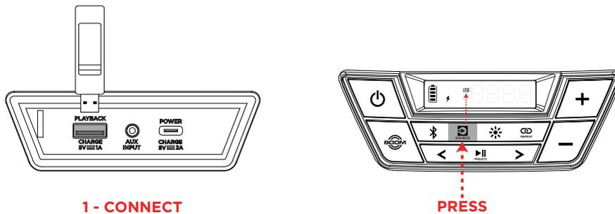
When a USB drive with compatible files is inserted into the **USB-A Playback / Device Charging Port**, Pathfinder™ Go will automatically switch to USB mode. If the USB drive has already been inserted and you are using another mode, press the **Source** button until USB mode is selected.
