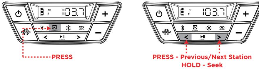
To use the radio, press the **Source** button so that **FM** is selected and shown on the display.
