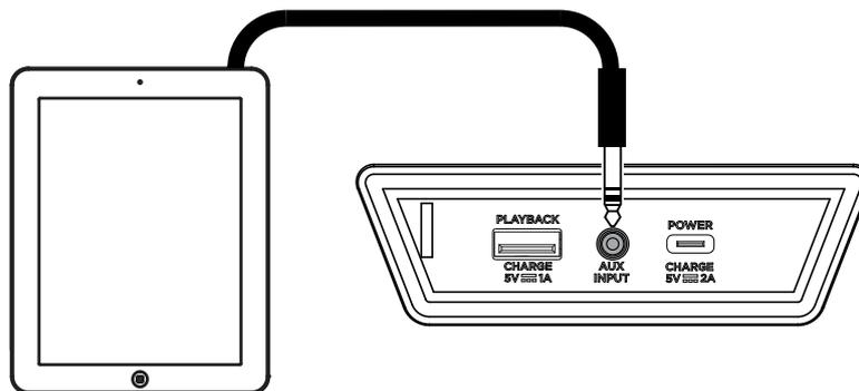
1. Connect a 1/8" (3.5 mm) auxiliary cable to the input on the rear panel of Pathfinder™ Go and connect the other end to an audio device such as an MP3 or CD player. The speaker will automatically switch the audio source to Aux mode but will maintain all Bluetooth connections.
