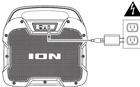
For the quickest charging time, power off Pathfinder™ Go and use the included USB-A to USB-C® cable to connect the USB-C® charging port on the rear panel of the speaker to a USB power adapter (DC 5V 2A, not included) connected to a power outlet, or your computer (powered on). A full charge can take up to 3 hours, depending on the specifications of your 5V, 2A adapter.
