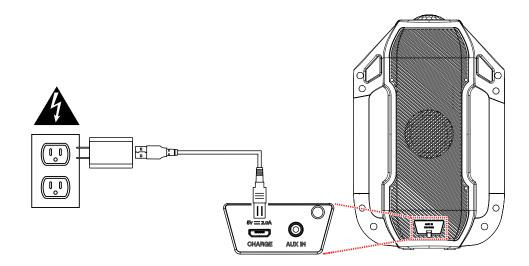
For the quickest charging time, power off Party Splash<sup>TM</sup> and use the included micro-USB cable to connect the micro-USB charging port on the rear panel of the speaker to a USB power adapter (DC 5V, 2A; not included) connected to a power outlet, or your computer (powered on). A full charge can take up to 4 hours, depending on the specifications of your 5V, 2A adapter.
