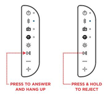
To answer an incoming call when connected via Bluetooth, quickly press and release the Play/Pause button. Bluetooth playback will be paused until the call is completed or rejected.
