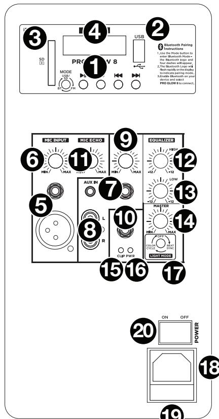
15. **Clip LED:** This LED will flash red if the signal from the inputs or media panel source is clipping. If this happens, decrease the setting of the **Mic Input Volume** knob, **Aux Input Volume** knob, or **Master Volume** knob.
